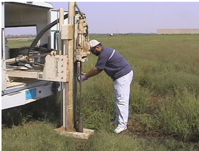
Plate 2. Drilling holes for ceramic cups installation.
