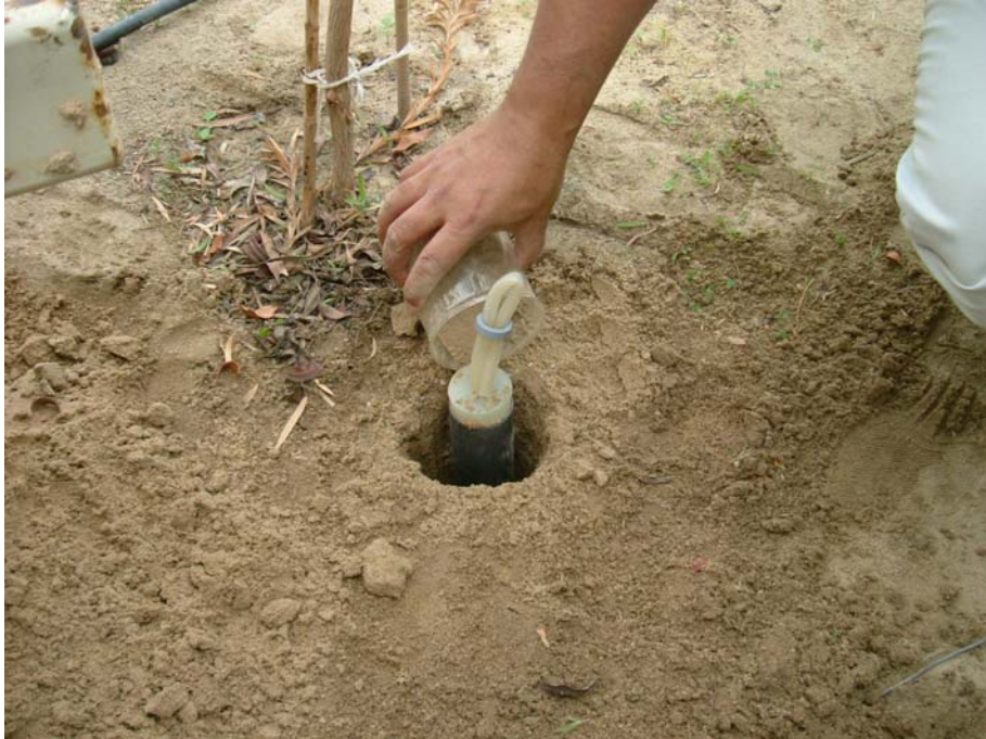
Plate 3. Installation of Ceramic Cups.
