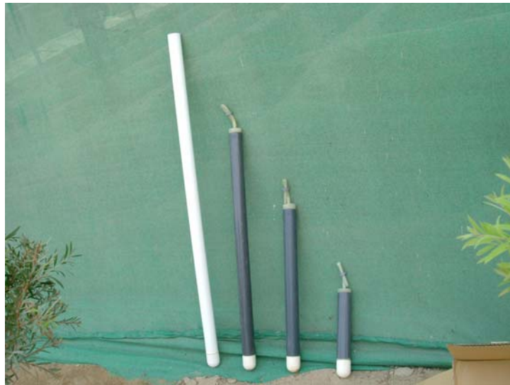
Plate 1. Ceramic Cups of Different Lengths Installed in the Study Area.
